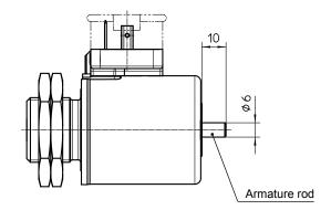
Fig. 11: Description in energised condition
