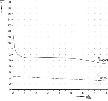
Fig. 4: Magnetic force-stroke-characteristic and return spring
