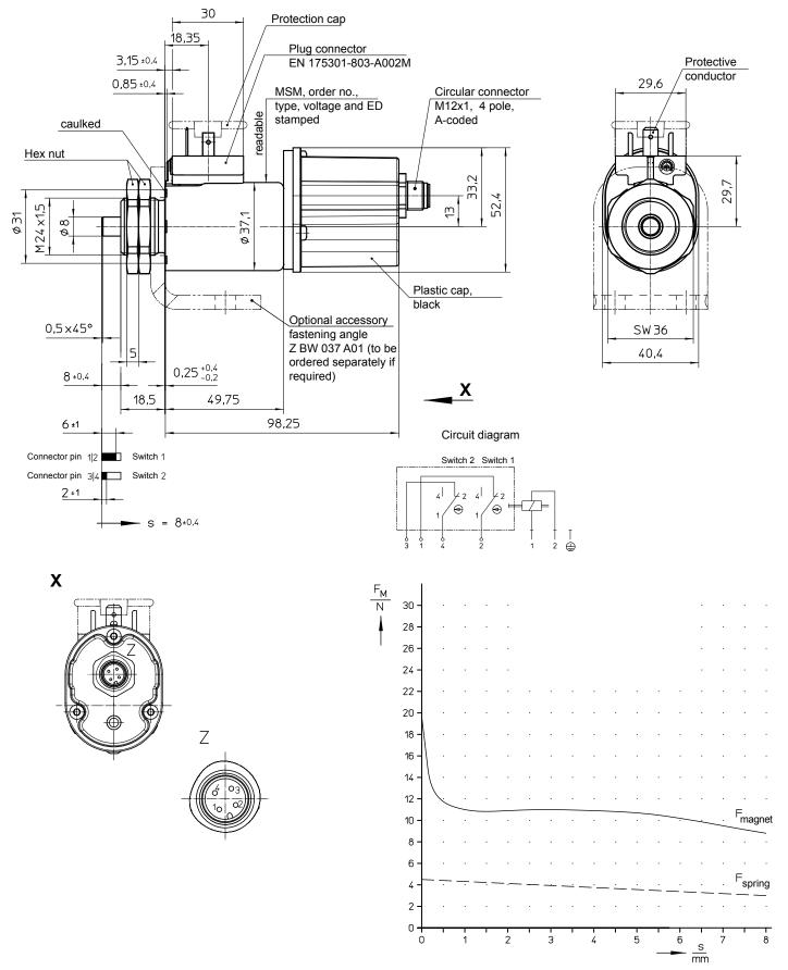
Fig. 8: Magnetic force-stroke-characteristic and return spring
