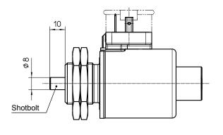
Fig. 14: Description in energised condition
