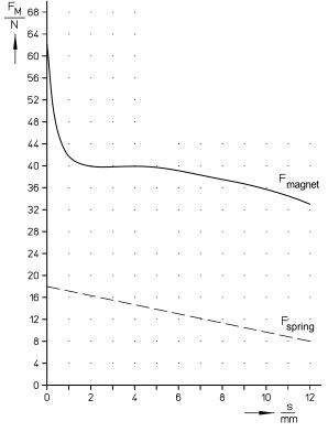
Fig. 22: Magnetic force-stroke-characteristic and return spring
