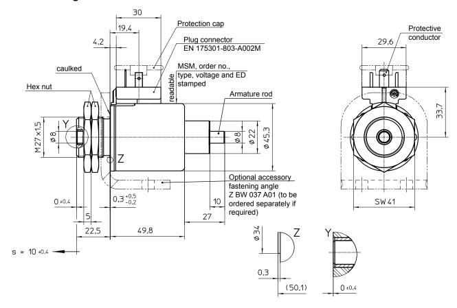
Fig. 13: Description in de-energised condition
