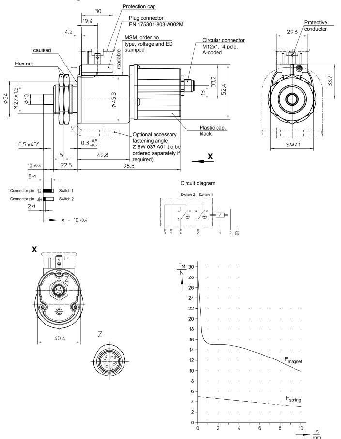
Fig. 16: Magnetic force-stroke-characteristic and return spring
