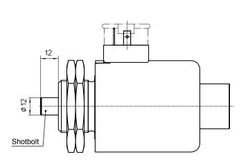
Fig. 21: Description in energised condition
