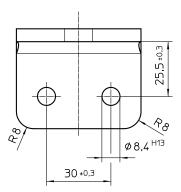
Fig. 26: Fastening angle Z BW 045 A01
