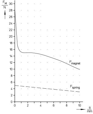
Fig. 15: Magnetic force-stroke-characteristic and return spring
