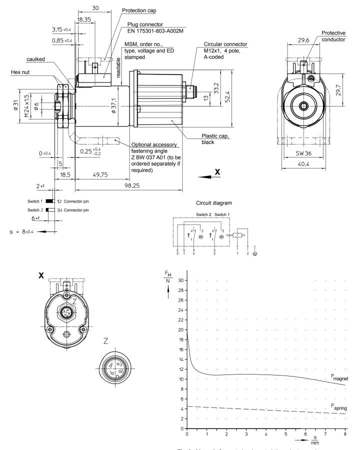
$\textbf{Fig. 9:} \ \ \textbf{Magnetic force-stroke-characteristic and return spring}$
