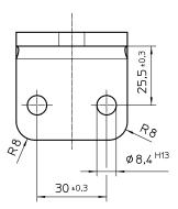
Fig. 25: Fastening angle Z BW 037 A01
