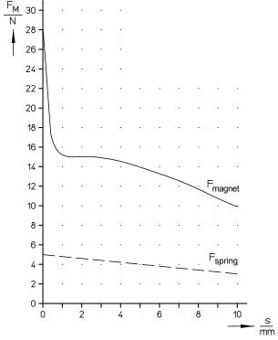
Fig. 12: Magnetic force-stroke-characteristic and return spring
