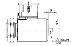
Fig. 3: Description in energised condition
