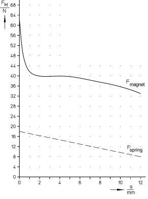
Fig. 19: Magnetic force-stroke-characteristic and return spring
