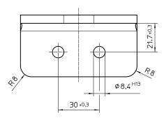
Fig. 27: Fastening angle Z BW 063 A01
