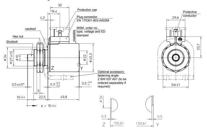
Fig. 10: Description in de-energised condition
