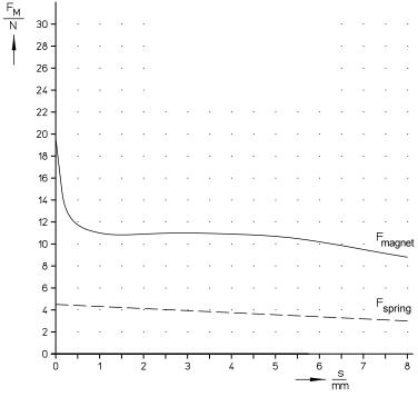
Fig. 7: Magnetic force-stroke-characteristic and return spring
