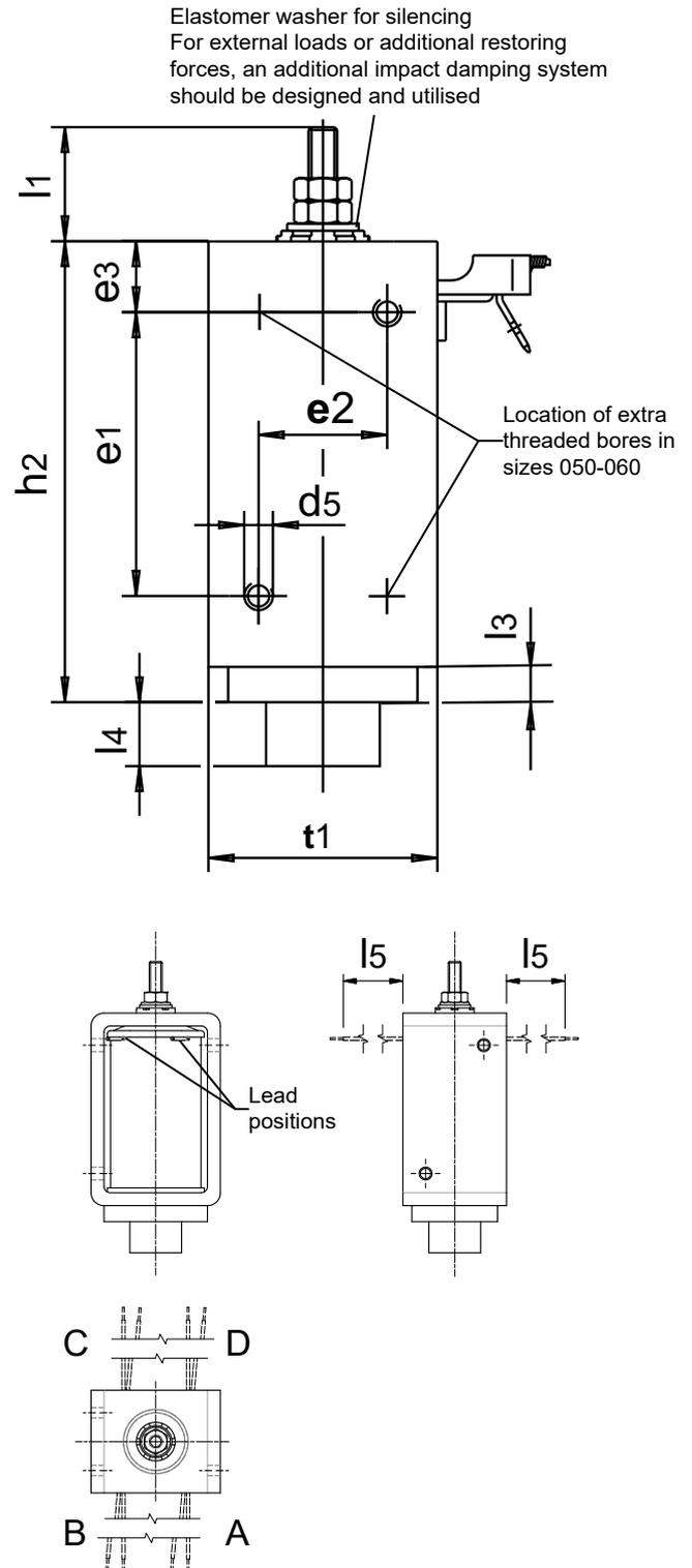
**Fig. 4:** Type G FC X... flying lead placement
